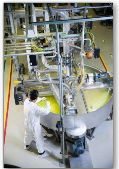
UO<sub>2</sub> Powder Production Capacity: 160 t/y UO<sub>2</sub>
