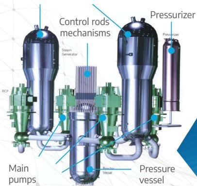
Steam dome (Self-pressurized) Control rods drives Steam generators (Secondary circuit) Control rods Core Pressure vessel CAREM INTEGRATED DESIGN
