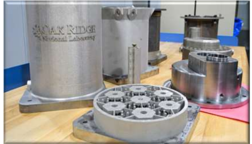
3D printed nuclear reactor components manufactured by Oak Ridge National Laboratory
