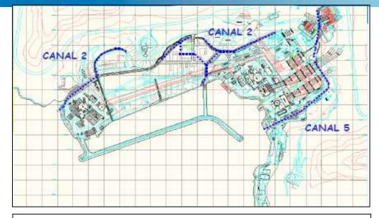
Flooding calculated considering rain fall of 10,000 years recurrence time (311 mm/hr)
