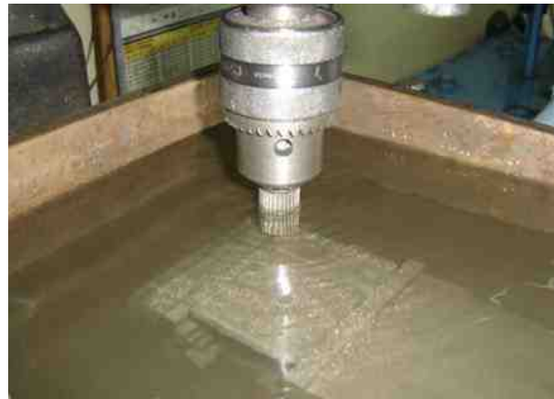
Flattening and cleaning of ingot through underwater machining
