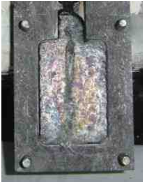
Ingot casting in graphite closed mould
