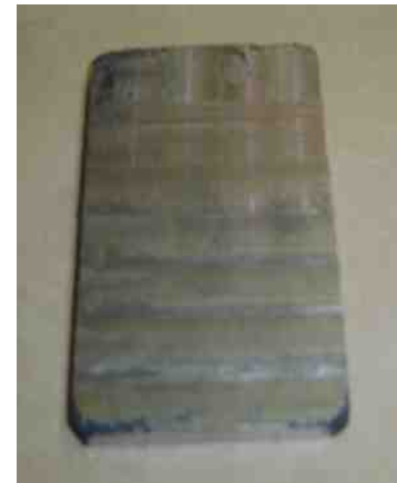
Flattening and cleaning of ingot through underwater machining
