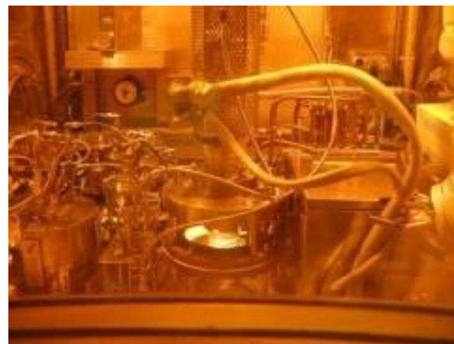
Severe Accident Fuel Test by HF induction Furnace in Shielded Cell
