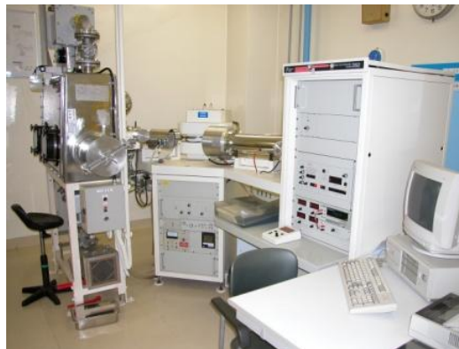
Thermal Ionization Mass Spectroscopy (TIMS) in GB for Isotope Analysis from Irradiated Fuel Solutions
