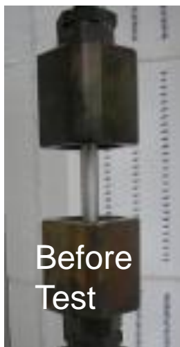
Tensile test for Irradiated Fuel Cladding
