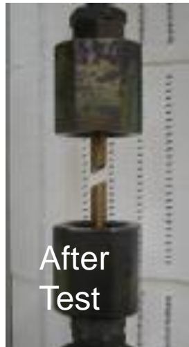
Tensile test for Irradiated Fuel Cladding
