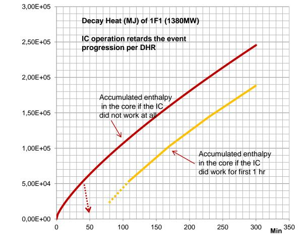
IC tank water decreased from 80% to 65%: ~50,000 to 60,000 MJ (a sum of latent and sensible heat)
