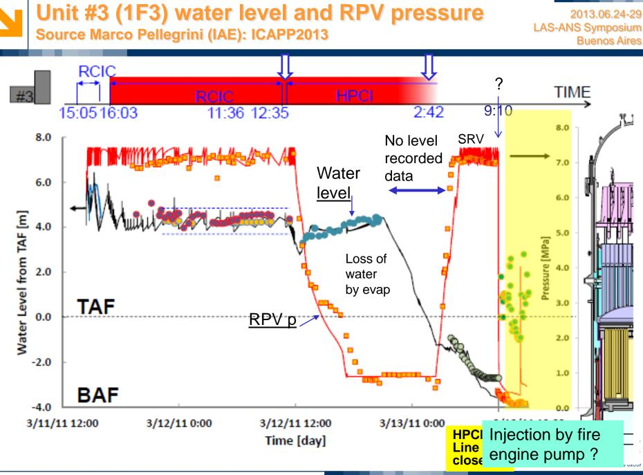
Before the reactor depressurized (March 13th around 9:00AM), as measurements show, the water level is already at BAF (= Bottom of Active Fuel).
