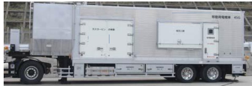
Alternate on-site AC power (Power vehicle)
