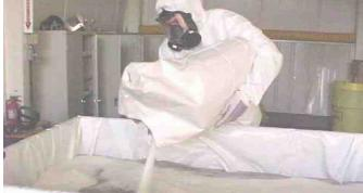
The polymer swells as liquid is added. More polymer is added to the top of the gel and then more
