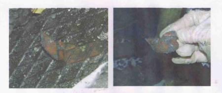
Figs. 7 and 8. Strippable coatings with metal oxides.
