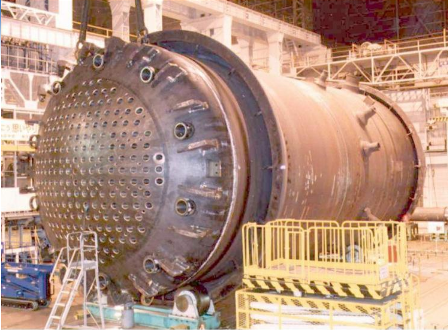
Photo.2 Fit up of Shell and Bottom Head
