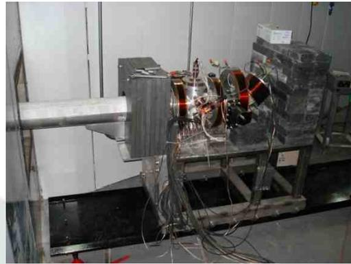
The positron beam-line partially inserted into the PULSTAR reactor's beam port #6.
