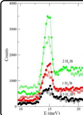
Neutron spectra of laser-produced single wall carbon nanotubes which are potential hydrogen storage materials. C.M. Brown, T. Yildirim, D.A. Neumann, M.J. Heben, T. Gennet, A.C. Dillon, J.L. Alleman, and J.E. Fischer
