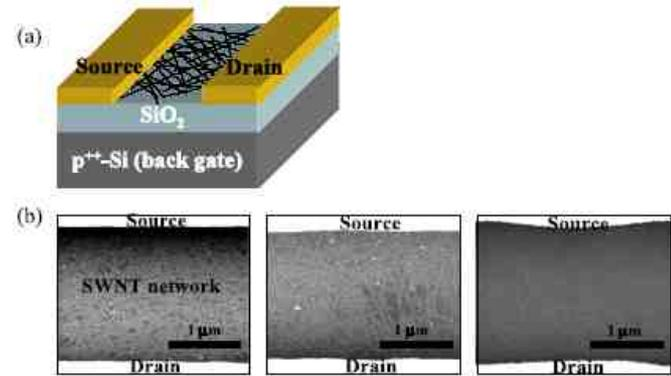
Figure 1. (a) Schematic drawing of single-walled carbon nanotube network field effect transistor (SWNT network FET), (b) SEM images of SWNT network FETs showing different densities of SWNTs connected between the source and drain electrodes.
