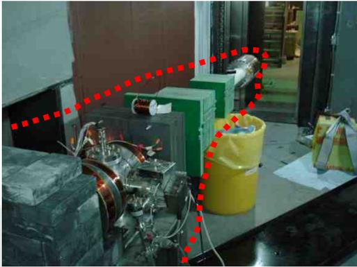
The positron beam-line (within the red border) prior to insertion into the PULSTAR reactor's beam port #6. The beam-line is ~15 feet long.
