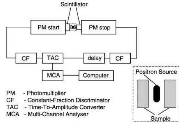
Figure 1 Principle of lifetime measurement: the source-sample arrangement is magnified.
