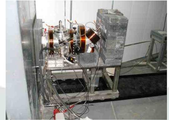
The positron beam-line fully inserted into the PULSTAR reactor's beam port #6.
