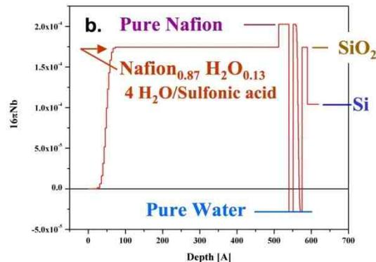
Neutron reflectivity data of water distribution within a model Nafion® PEM fuel cell membrane. Dura, J.
