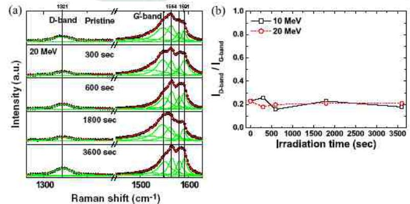
Figure 5. (a) Raman spectra at an excitation wavelength of 633 nm for the SWNT network FETs before (pristine) and after proton irradiation of 20 MeV for 300, 600, 1800, and 3600 s corresponding to the fluence of  $1.2 \times 10^{11}$ ,  $2.4 \times 10^{11}$ ,  $6.9 \times 10^{11}$ , and  $1.4 \times 10^{12}$   $\text{cm}^{-2}$ , respectively. (b) The intensity ratio of D-band to G-band at different radiation time periods for 10 and 20 MeV proton beams.
