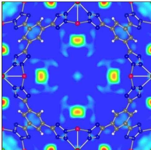
Hydrogen molecule adsorption sites (red-yellow regions) in Mn-BTT (Mn - 1,3,5 benzenetristetrazolate) determined by neutron diffraction. This material is a metal organic framework candidate material for hydrogen storage. M. Dinc; A. Dailly; Y. Liu; C.M. Brown; D.A. Neumann; J.R. Long
