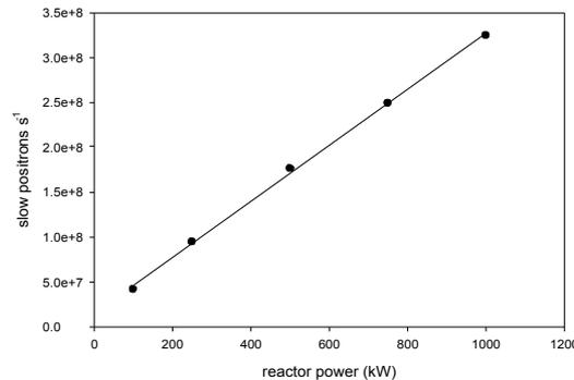
Recent results of positron generation by the PULSTAR reactor using the positron beam-line shown above. The results indicate a beam intensity exceeding  $3 \times 10^8$  e<sup>+</sup>/s at full reactor power (1-MW). On-going modification to the beam-line are expected to raise this number substantially. The figure on the left shows the signal of e<sup>-</sup> - e<sup>+</sup> annihilation (i.e., 511 keV gamma-rays) in the detector.
