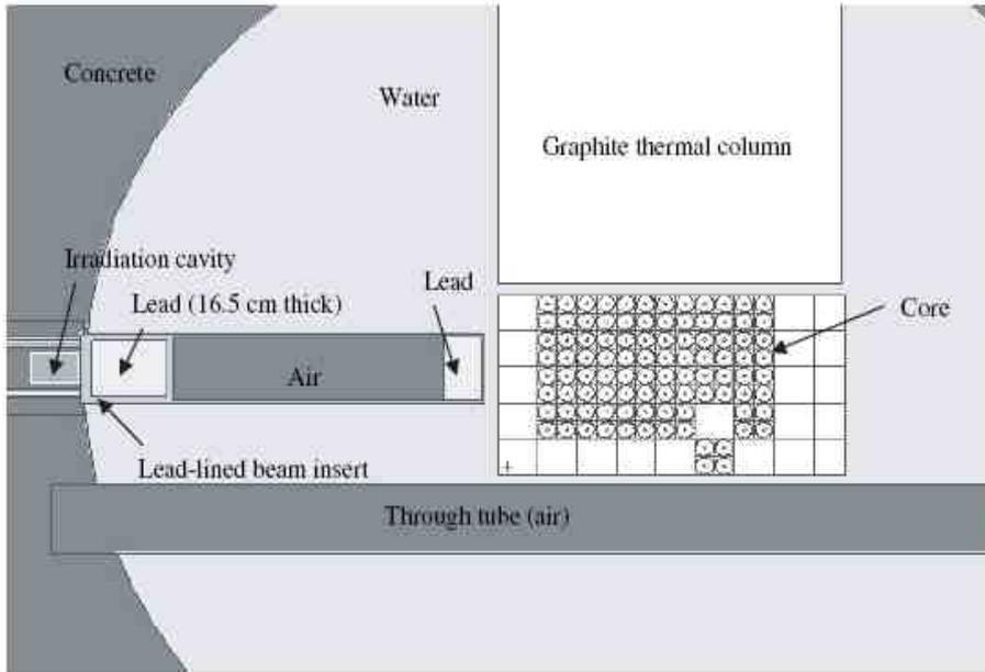
Figure 1. The two-dimensional MCNP model of the MUTR core and the irradiation beam port.
