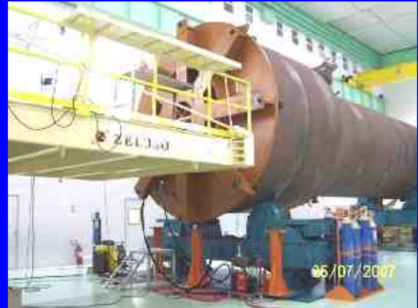
Helium leak test
