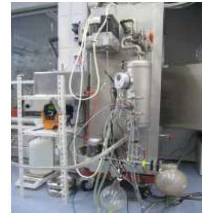
Molecular Sieve Test facility of TÜV Organic Iodine Retention Test
