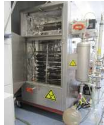
Molecular Sieve Test facility of TÜV Organic Iodine Retention Test
