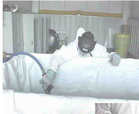
The waste is pure liquid and contains contaminants of radioisotopes. About 100 lbs of *Waste Lock*® is first added to the bottom of the box.
