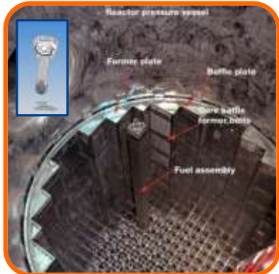
Baffle Bolt Replacement
